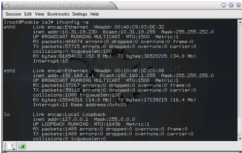
Illustration 14 On the Linux box: results from “ifconfig -a” command
