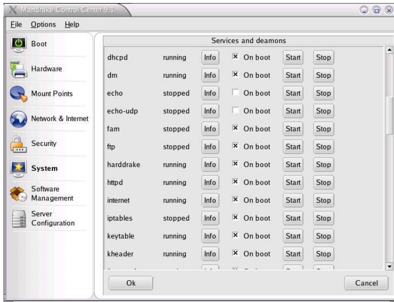
Illustration 20 Verifying if the DHCP daemon is running and startup configured correctly.
